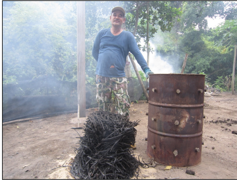
Figure 4. Charcoaling of Bamboo residue twig by single drum kiln
